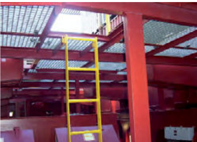
Bottom: GRP gratings installed on a ship
